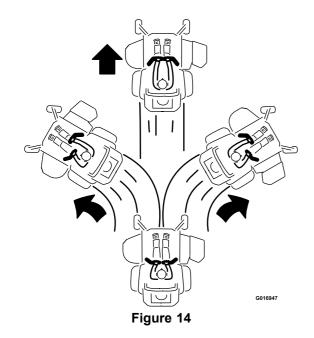
To turn left or right, pull the motion control lever back toward neutral in the desired turn direction.
